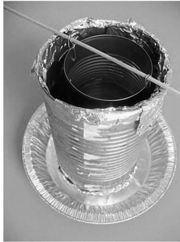
Figure 2. Arrangement of the cans and wrapping inside of the larger can with aluminium foil
